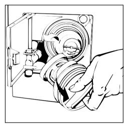
■ Turn the drain pump impeller (in the back of the chamber) by hand to check that it rotates freely. Any foreign objects should be removed.
